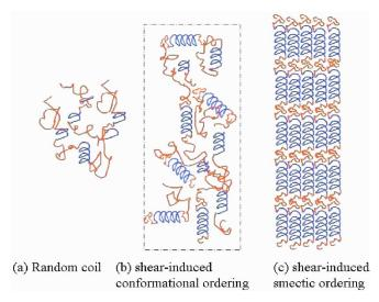
FIG. 4 (color online). Schematic picture of the process of shear-induced ordering of smectic bundles. The density modulation of the smectic layers consists of alternating rigid helices and flexible disordered segments.
