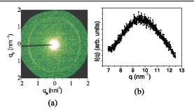
FIG. 2 (color online). Two-dimensional SAXS pattern of iPP displaying smectic ordering at 200 °C (a) and corresponding one-dimensional WAXS pattern (b) after a steady shear with shear rate 1 s<sup>-1</sup> for 2 min.
