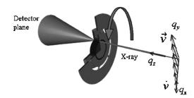
FIG. 1. Scattering situation in the shear geometry used with reciprocal space picture of the scattering wave vector  $\vec{q}$ , where  $q = 4\pi \sin\theta/\lambda$ ,  $\lambda = 0.154$  nm is the x-ray wavelength, and  $2\theta$  is the scattering angle.
